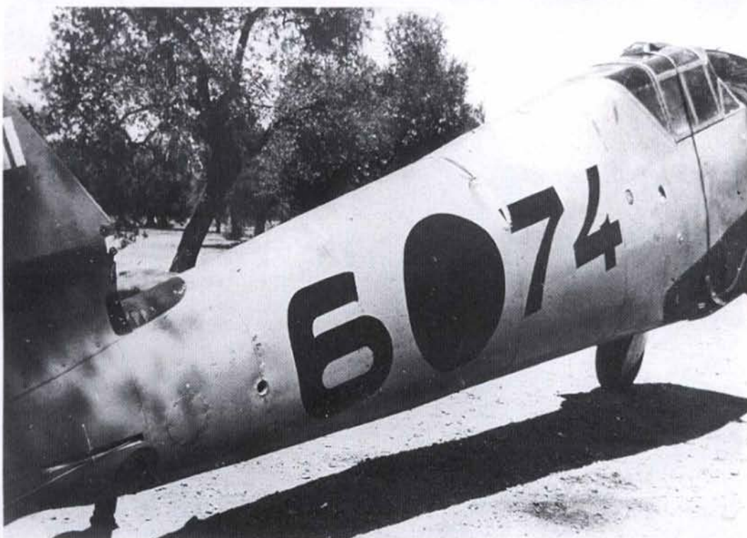
194: This Bf-109D, 6-74, was most probably being scrapped (the wings and tailplane are already off) after major structural damage to the fuselage spine which has been broken, probably due to a combat overstress. The place seems to be La Cenia, the time being summer 1938. The dark areas of paint left where the flying surfaces have been removed are note worthy
