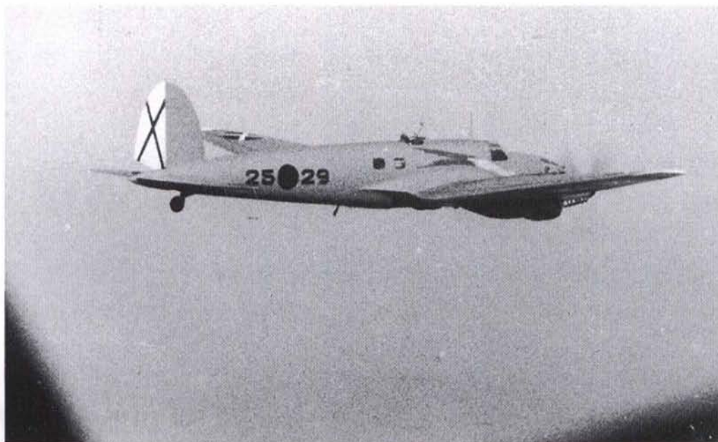
311: A comet bearer, He 111B-1, 25-29, of I.K/88 flying towards enemy territory, as seen from a wingman's pilot's point of view. Note that the exhausts are of the first 'organ pipe' style and the ventral gun tub is retracted. The overall effect is of a very clean grey machine. The picture is believed to have been taken on 17 December 1937 when the aircraft, based at Burgo de Osma, were attacking troop concentrations at Teruel
