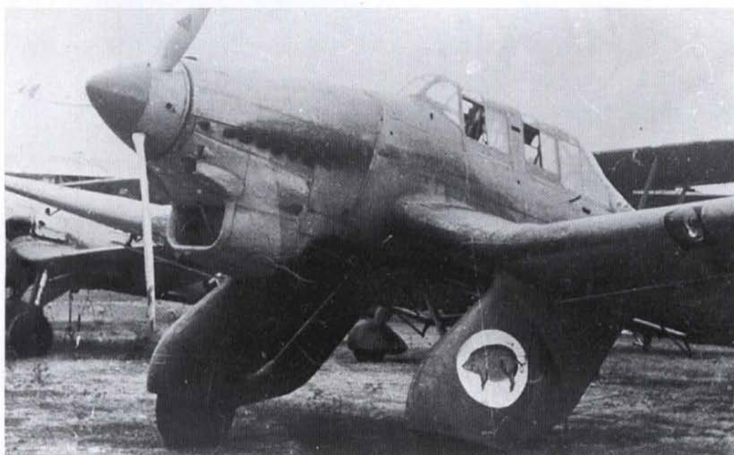
371: The war is just over and all the combat aircraft are gathering in Madrid for the final victory parade. Among other types of aircraft (see a He 70 at left, and the spatted undercarriage of a Hs 126 between the Stuka's wheels) is this Ju 87A, which is not 29-2 (no antennae) nor 29-3 or 5 (see different splinter scheme on the nose), from which we may conclude it is 29-4, the usual mount of the leading crew, Lt Haas/Fw Kramer. Note the stain over the engine exhaust and the presence of the little pig emblem
