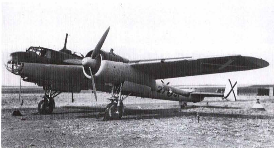
43 Above: A view of 27-29 which shows the Bramo radial engines of the Dornier Do 17P to advantage. These later models also received the devils head emblem on their cowlings
