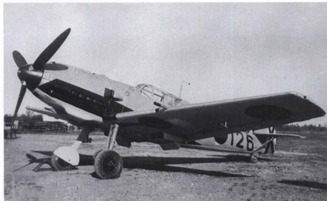
206: This is Bf109E-3 6-126 at Prat de Llobregat during World War II, in immaculate condition and wearing a slightly different finish to which it was delivered. The main difference between the E-3 and earlier models was the pair of 20mm MG FF wing cannons
