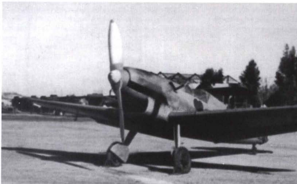
408: This is the Messerschmitt Bf 109 V3 as flown by Hannes Trautloft who has had the green heart emblem applied to it as a reminder of his origins in the 'green heart' of Germany. The aircraft has a large wooden propeller and appears to be still in a natural metal finish
