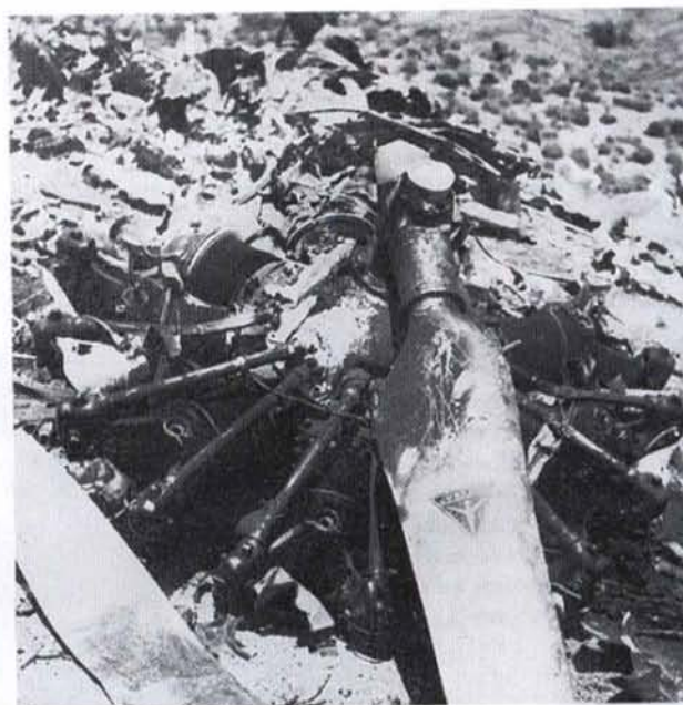
267: Auntie Ju was a strong lady. The corrugated construction of the Junkers Ju 52 meant that it could survive impacts like this (a mid-air collision?) and still get home
