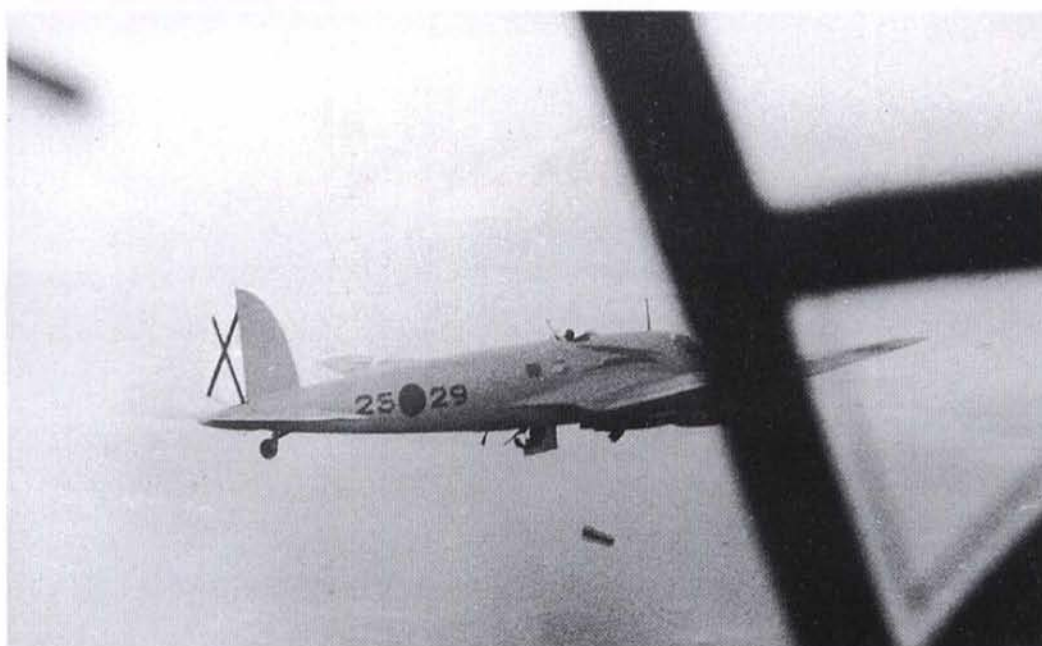
313: Actual combat footage from Spain is rare, but here we have He 111B-1 25-29 over the target at the point of bomb release. The dorsal gunner can be clearly seen and the ventral gunner's tub has been extended and manned. This was the most vulnerable phase of the flight when it was necessary to fly straight and level to allow the bomb aimer to carry out his job, but this also presented a good target to enemy fighters. An SC 50 bomb has just left the bomb bay, tailfirst, and is aligning itself into the correct position
