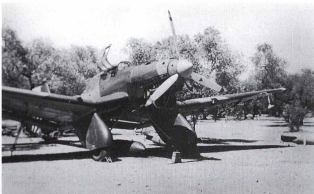
369: Same scene as in photo 368. One can see the oil can under the nose of the aircraft, and the main bomb lying on the ground, between the undercarriage legs. The cockpit was left open at all times in Spain, in order to limit the excessive heat of the summer
