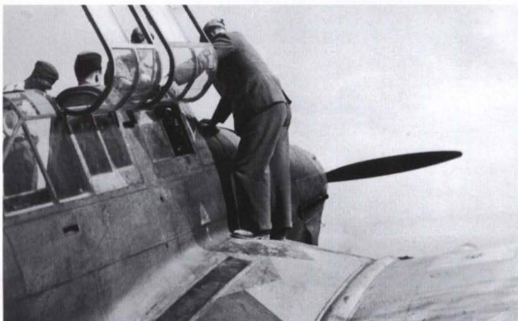
370: Something seems to be baffling the ground crew. Note how the upwards hinging canopies restricted access to the cockpit, the non-slip walkways on the wing root, the reinforcing plate over the wing joint and the splinter camouflage
