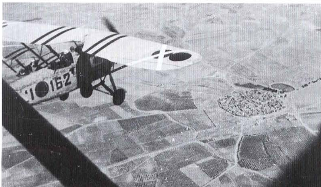
74: He 46C 11-162 sports a curious camouflage scheme where the upper fuselage has a mottle over the grey background, but nothing has been applied to the generous wing. The picture is also illustrative of the distance between aircraft in a formation, as a third 'Pava' can just be seen under number 162. A small village enclosed by a wall and surrounded by fields can be seen down below
