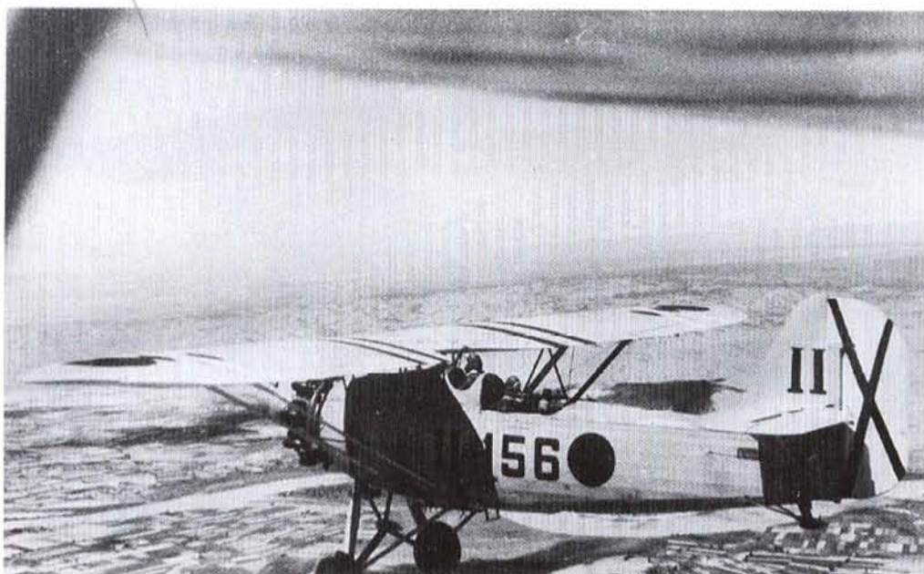
68: Most of the He 46Cs were used in standard RLM light grey 63 (L40/52) livery, like here with 11-156 and 11-157 below. Noticeable is the first style of registration, with both the type number and aircraft number painted before the black fuselage disc. This was later changed by putting the cockade between them.
