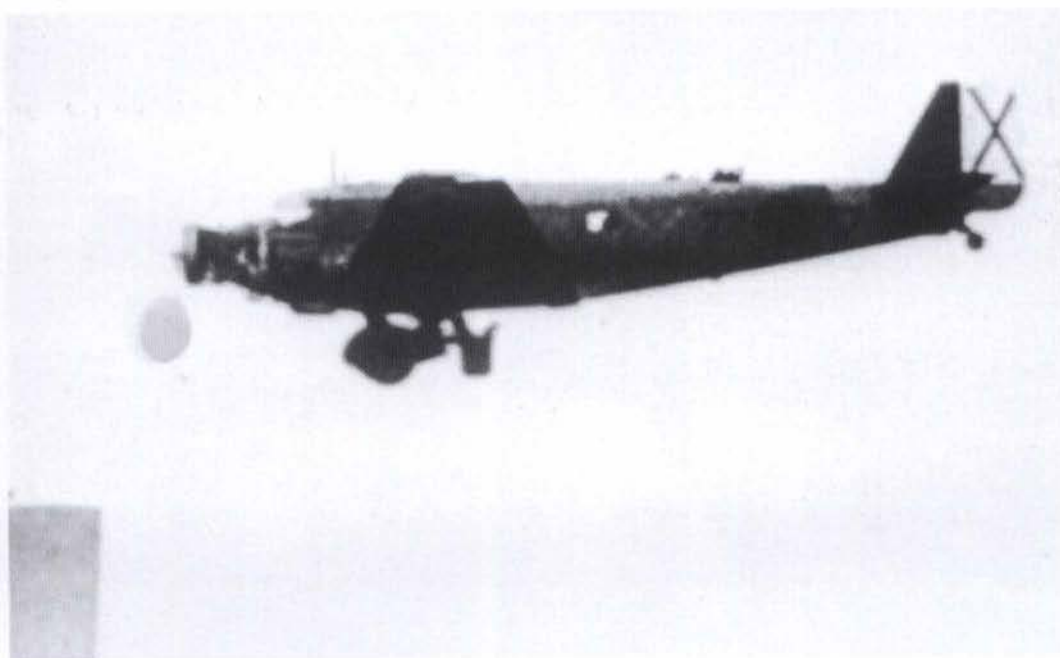
247: Extracted from actual film footage taken on operations by propaganda crews. This shows 22-87 of 2.K/88, another dedicated bomber, over the target with its ventral gun tub extended. The drag was so significant that it was the custom only to use the device when enemy fighters were expected
