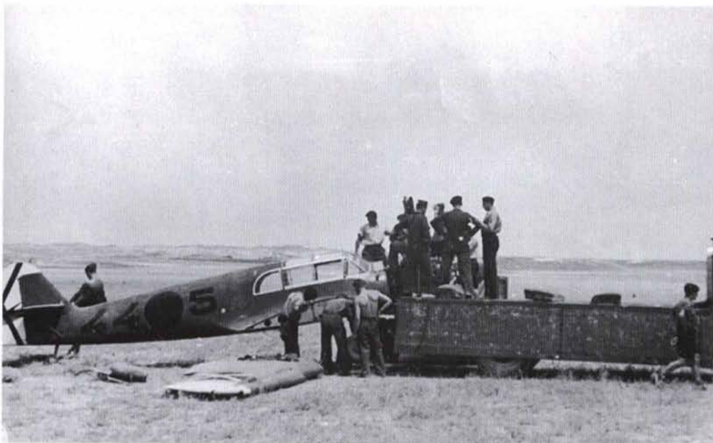
426: After disassembling the wings, the salvage team has lifted the whole aircraft on a medium truck. There are at least ground crewmen working on the operation
