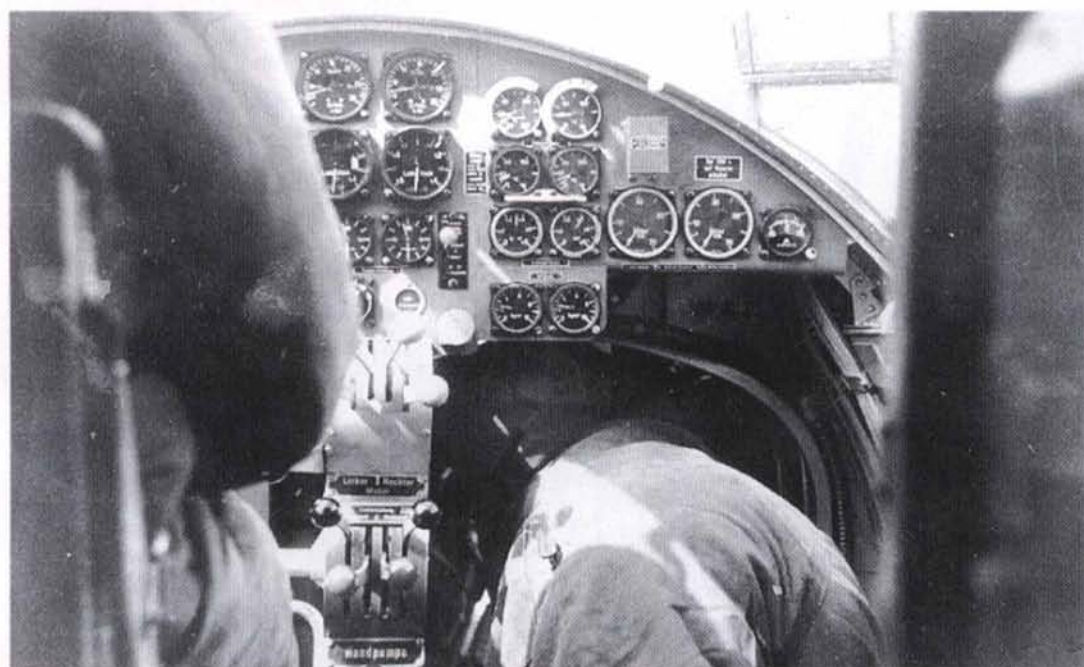
338: The bomb-aimer of an He 111B moves to his station while the pilot scans his instruments. The main interior finish appears to be RLM 02
